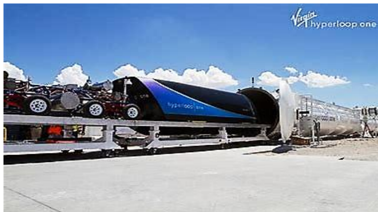
Kapsula ∞ XP-1 uvlači se u testnu cijev Picture Credits: hyperloop-one.com
