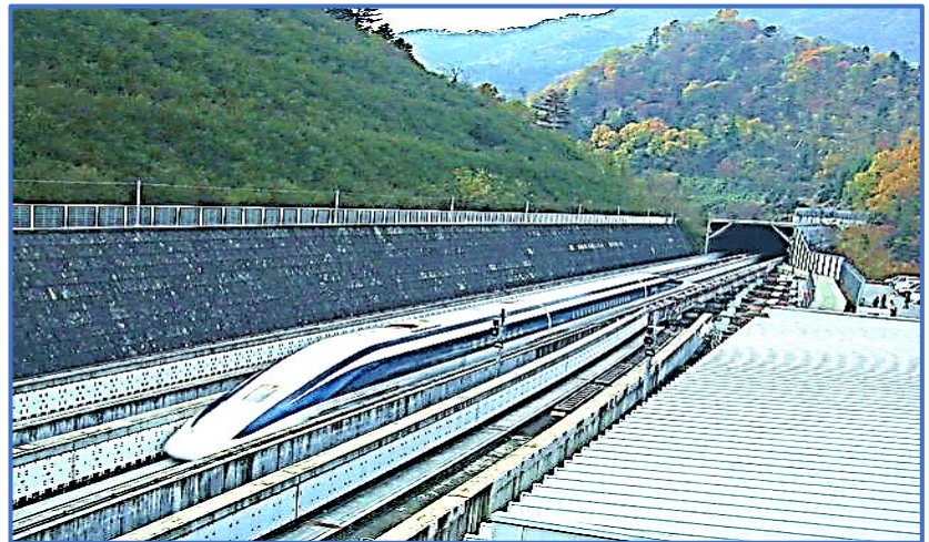
JR Central SCMaglev vlak rabi 'null flux super-conductor magnet-base' - Credits: Yosemite - Own work, CC BY-SA 3.0
