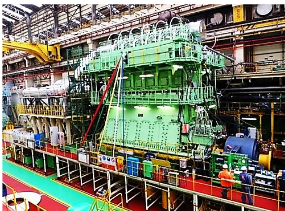
The first IMO Tier III compliant Wärtsilä X72 diesel engine with pre-turbocharger SCR passed its shop test on 23rd March 2016.
