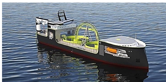
The Ulstein LX109 combines the 'Cable Arch' concept with the X-Bow and X-Stern
