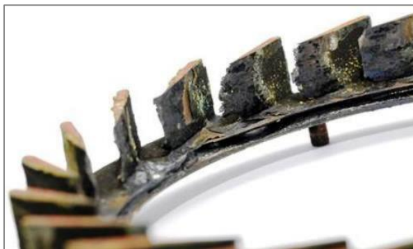
Oštećeni sapnički prsten - Image credit Tru-Marine marinediesels.info
