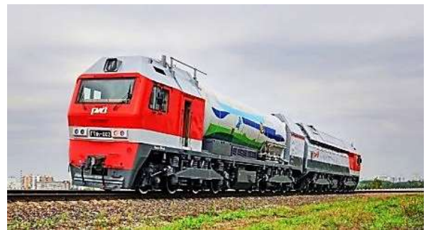
Lokomotiva s plinskom turbinom (Image: Gazprom)
